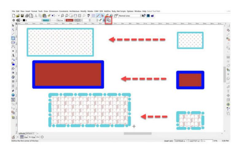
**Pick Point Hatch** – Pick-Point-Hatch now works with gaps in 2D objects. For example, trying to fill an area bounded by a Polyline, when there are gaps in the Polyline. Improvements to pick-point also apply to ADT objects (Walls, Doors and Windows), allowing to similarly fill in gaps between these objects.
